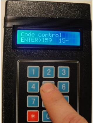
Fig. 9 shows that the user has entered the coding setup. In order to start manual coding enter 1; 5; 9;.
