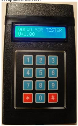
Adaptation module has a keyboard, which is used for data input and controlling the device itself, LCD display, on which the information is displayed and an OBD connector that is used to connect the vehicle to the module.
